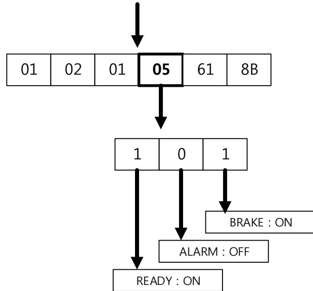
3) Example of parameter reading for 0x0020~0x0023
