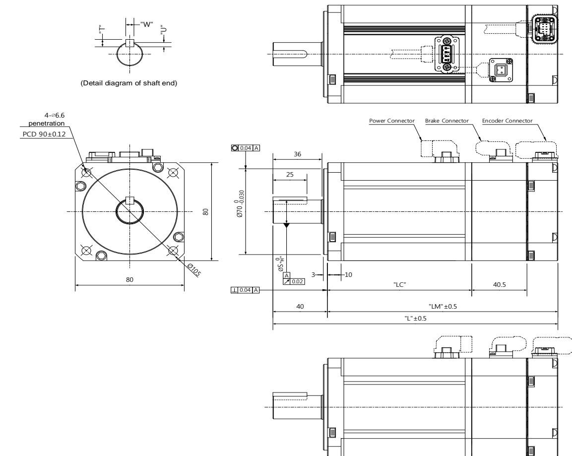
&lt;When the cable withdraw direction is the opposite of the shaft&gt;
