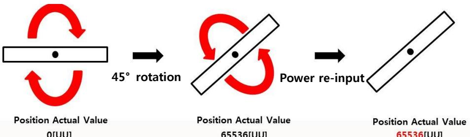
When you set the value to 2, power re-supply resets the multturn value to 0[revolution] but brings the encoder's singleturn value for the current position and displays it.
