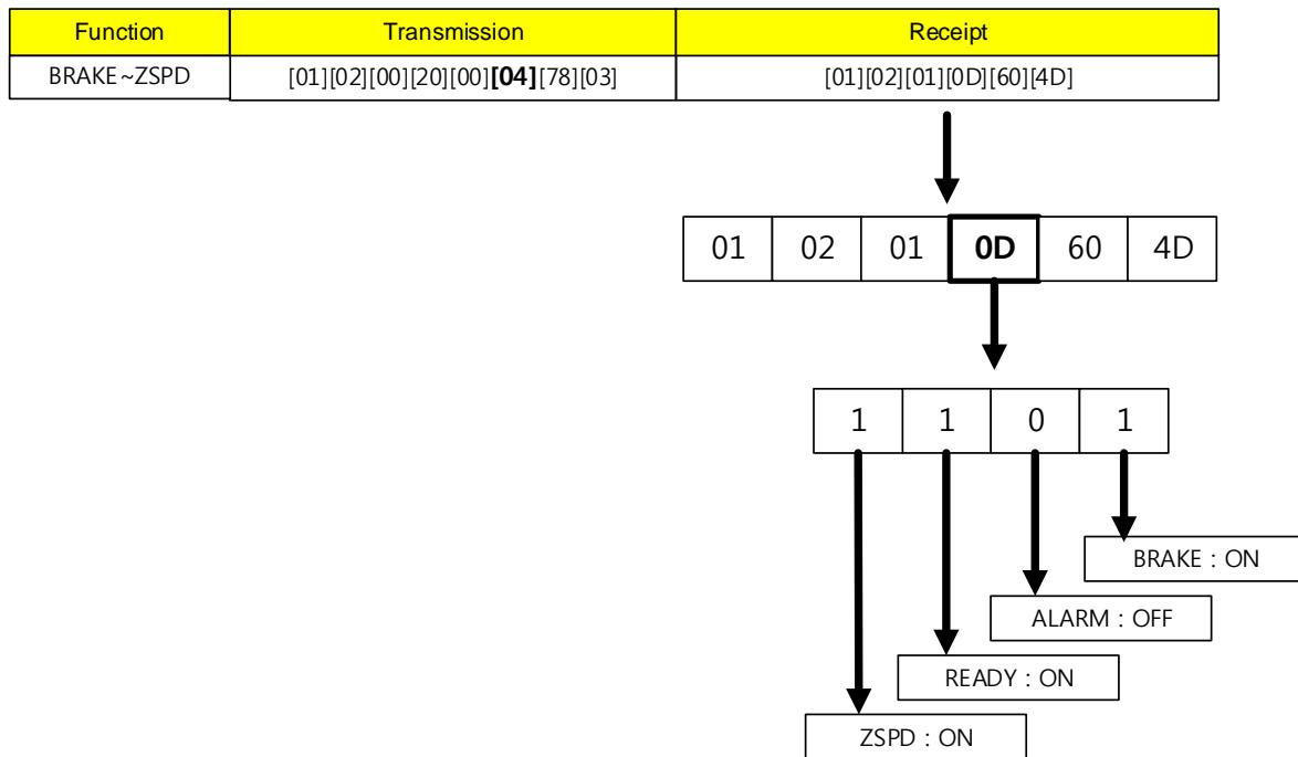
4) Example of parameter reading for 0x0020~0x0024
