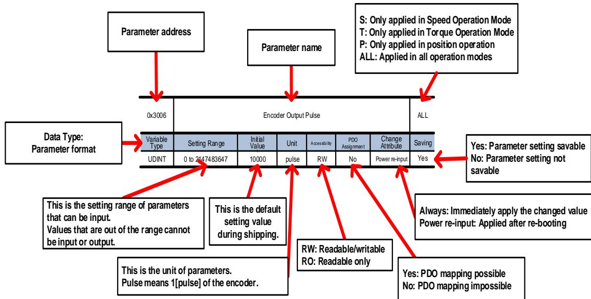
Parameters are categorized into immediately applied ones and ones that can be applied only if the servo power is turned on/off. The above table provides an example of the variable attributes.
