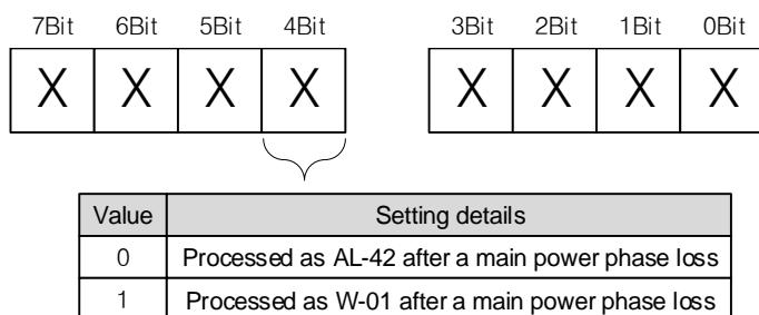
The 4th bit determines the servo's state in the event of a phase loss of the main power.
