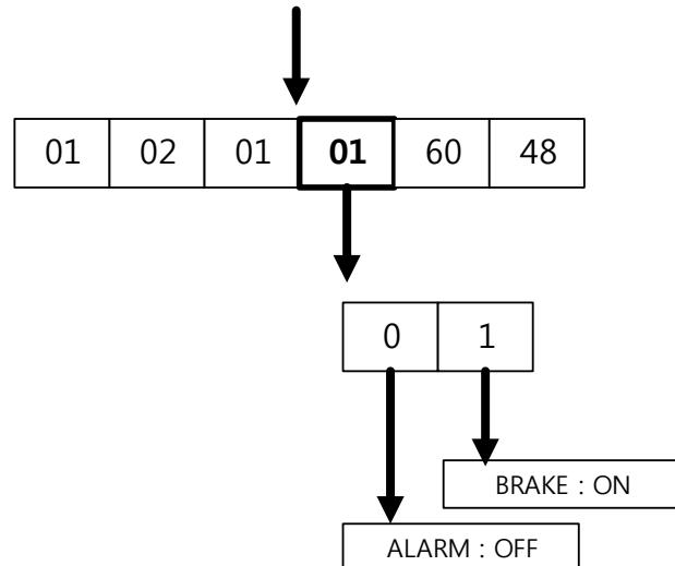
2) Example of parameter reading for 0x0020~0x0022
