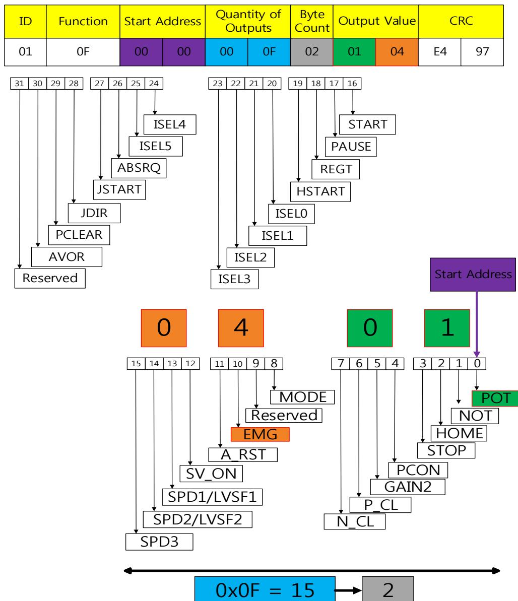
When you assign 15 Quantity Of Outputs while starting from 0x00 for the starting address, you can control the input up to 0x14. As the upper and lower Output Values are swapped, please be careful when you input them. When you input '01 04', for example, they will be swapped into '04 01'. 04 will turn on EMG, the 10th bit, and '01' will turn on POT, the 0th Bit.
